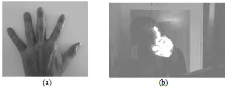
Fig. 4 - The scanned forefinger (a) and position of forefinger during scanning (b)
